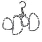
6. Adjust the tension of the curved arms so that they hold the can firmly when they are pushed onto the can.
